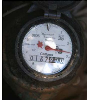
The small star wheel is used to detect leaks and minor usage. The odometer reads total gallons used. Read the odometer left to right, including the fixed zero on the far right.
