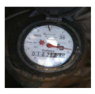
Step 3. Take the lid off the meter box and lift the protective cover. See "How to Read Your Water Meter" pamphlet for directions. Watch the meter. Your meter will have a red star wheel that is commonly called a "leak indicator." If it is spinning, even very slowly, you have a leak. If it is not spinning, look at the red pointer and note the number it is pointing at.
